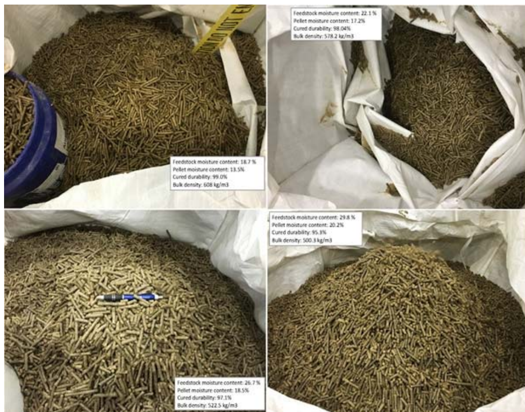
Figure 15 Photograph of corn stover pellets produced at high moisture contents
